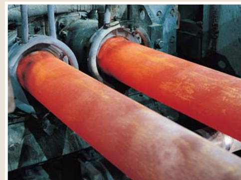
수평연속주조 _ Horizontal Continuous Casting
